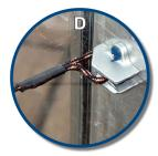
Above are images of the results of LifeLine testing in Canada. As the explosion progresses, you can see in (B) that the sheet of glass has been separated from the frame and is beginning to fold around the shock chords. (C) As the LifeLine cords absorb the blast energy, they effectively prevent the filmed glass from entering the building. (D) Close up of the LifeLine attachment point.
